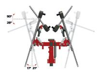
Independent hydraulic tilting of vertical and horizontal bars for working on slopes.
